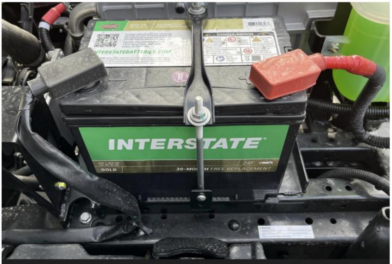
Figure 1 OEM 12v 750 CCA Start Battery located under the Cab
