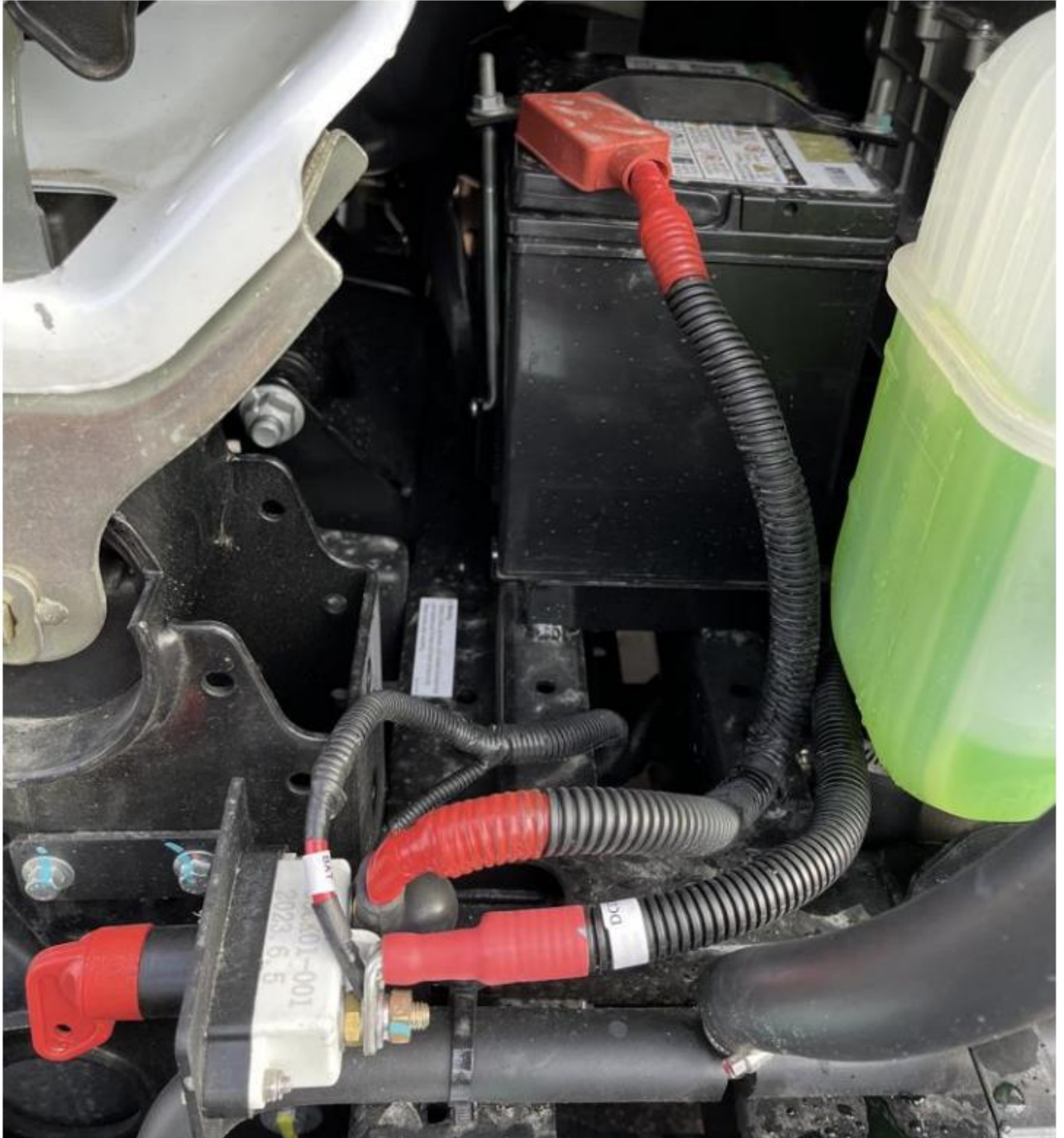
Figure 2 OEM Chassis 'Master Switch' located just aft of Cab. (D.C. + / - terminal connection posts)
